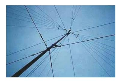
1,5 - 30 MHz Frequency range Impedance 50 ohm **VSWR** < 2,5 (DIAG. 1) Polarization HOR. 1 kW CW Maximum power Radiation diagram DIAG. 2, 3 Height 10 m Lenght of sections 7 X 1,4 m Mass of antenna 67 kg Section diameter 60 mm 30 min./3 Mount. time/no. of pers. Mounting area 25 m Wind velocity 120 km/h Temperature range -40....+70 °C
