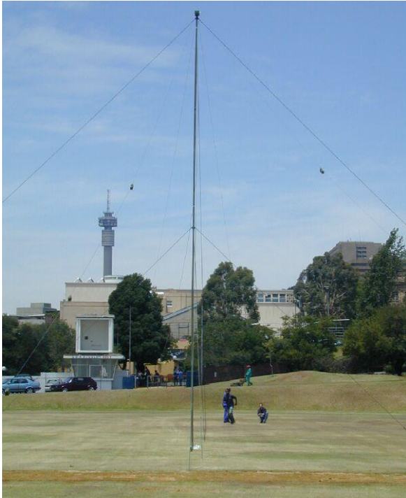
Antenna mounted on 10 m mast
