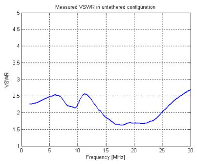
Figure 1: Measured antenna VSWR in untethered configuration
