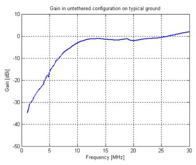
Figure 2: Antenna gain in untethered configuration
