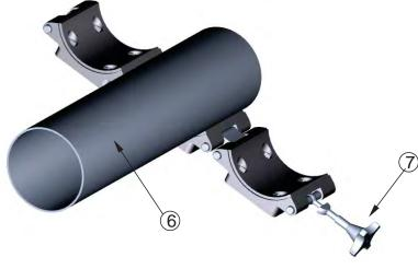
TRIVAL ANTENE already delivered hundreds of such clamps to many of our customers around the world. Clamps are mainly used for transportation purposes on the top of the vehicle/shelter as well as for the vertical attachment of the mast asside of the vehicle.
