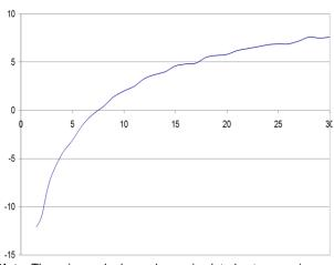
**Note:** The gain graph above shows simulated antenna gain over "average" ground with conductivity of 0.005 S/m and relative permittivity 13 and takes into account ground losses as well as resistive losses in the antenna.
