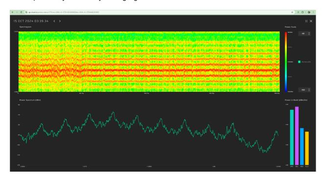
The system classified this event as 100% jamming across all visible GNSS constellations, with no spoofing signatures detected.
