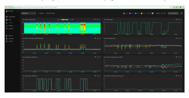
This interference had a high-power pulsed nature, repeatedly turning on and off.
