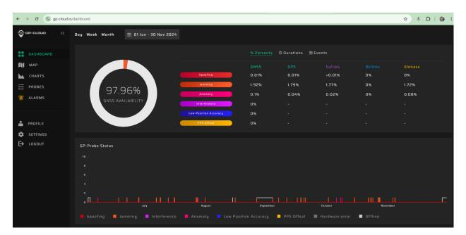
Over the six-month observation period, GNSS signals remained available with the required quality for 97.96% of the time, meaning that only 2.04% of the collected data was affected by interference, data anomaly or signal quality degradation.
