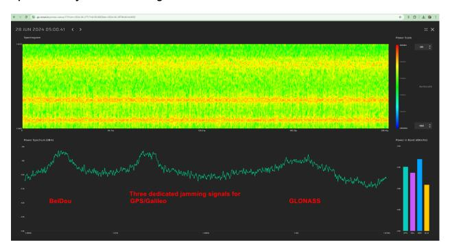
Spectrogram analysis revealed that the jamming signal had a complex structure, consisting of three distinct interference components targeting:
