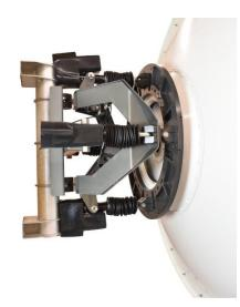
The LinkAlign-15LPT-40 is an antenna positioner designed from the ground up to automatically maintain microwave line of sight communication links for 4-6 ft antennas. Narrow beam antennas often require realignment due to seasonal fading of misalignment caused by wind loading.
