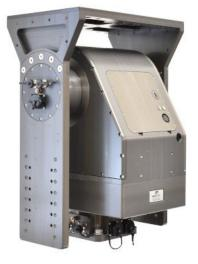
The LinkAlign-360FER-56 is a Power Over Ethernet (PoE) antenna positioner designed from the ground up to automatically point and peak directional antennas for microwave Line of Sight and satellite communications. Satellite applications include geo stationery positioning and inclined orbit tracking.
