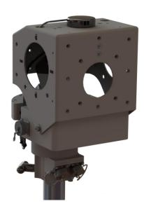
The LinkAlign-360RPT-F10 is a Power Over Ethernet (PoE) antenna positioner designed from the ground up to automatically point and peak directional antennas for microwave line of sight communications. The LinkAlign-360RPT-F10 is unique from the LinkAlign-360RPT-10 in that the base of the positioner containing the PoE input and ethernet pass thru connectors does not rotate relative to the mast, eliminating potential cable wrap challenges.
