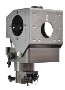
The LinkAlign-360RPT-F20 is a Power Over Ethernet (PoE) antenna positioner designed from the ground up to automatically point and peak directional antennas for microwave line of sight communications. The LinkAlign-360RPT-F20 is unique from the LinkAlign-360RPT-20 in that the base of the positioner containing the PoE input and ethernet pass thru connectors does not rotate relative to the mast, eliminating potential cable wrap challenges.
