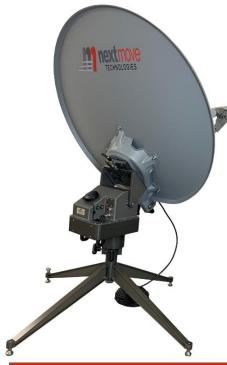
Satellite communication becomes an important part for any state or local emergency operation plan when terrestrial communication such as cellular is unavailable or goes down during natural or manmade disasters. The LinkaSat-90-Ka-HN is a lightweight auto acquire satellite system designed to work with Ka Band HughesNet Business Class Service to quickly get your team back online.
