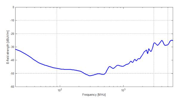
Simulated E-field strength required for 12 dB NF receiver, 1 Hz bandwidth and 0 dB SNR (includes external noise in urban environment)
