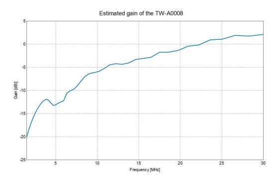
**Note:** The gain graph above shows simulated antenna gain over "average" ground with conductivity of 0.005 S/m and relative permittivity 13 and takes into account ground losses as well as resistive losses in the antenna.
