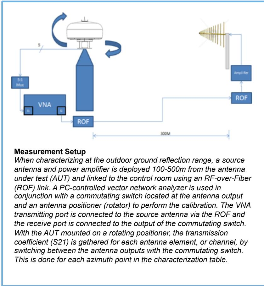
During characterization, it can be helpful to use source setups that provide cross-polarized waves, and with the waves originating from different elevation angles, to see how the antenna characterization table performs under stress.
