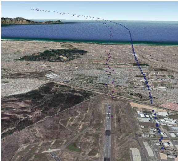
MLAT measurement highlighting the occasional inaccuracies of ADS-B
