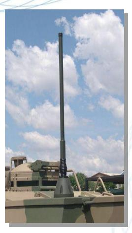
The VCF115-512 mobile antenna is an omnidirectional, vertically polarized, rugged and versatile V/UHF antenna intended for ground to air, ground to ground, ship to shore, marine and general tactical mobile communications in the 115-512MHz range.
